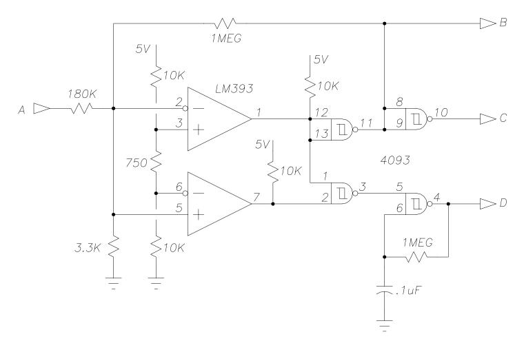
This circuit senses a voltage on point "A". If it is above 145VDC or below 135VDC then step pulses are output on point "D". If the voltage on "A" is above 145VDC then point "B" is +5VDC, otherwise it is 0VDC. Point "C" does the opposite of "B". Either "B" or "C" may be used as direction outputs.
